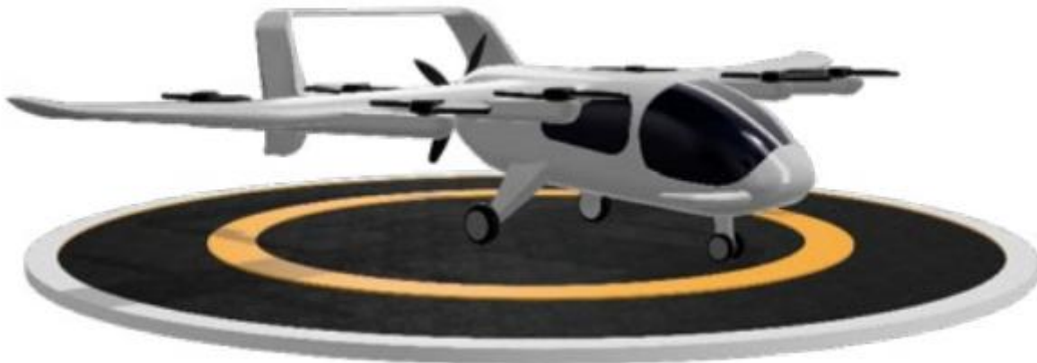
Figure 4: Example of a lift + cruise VCA
