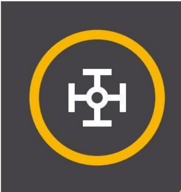
FAA broken wheel marking EASA V on blue marking
