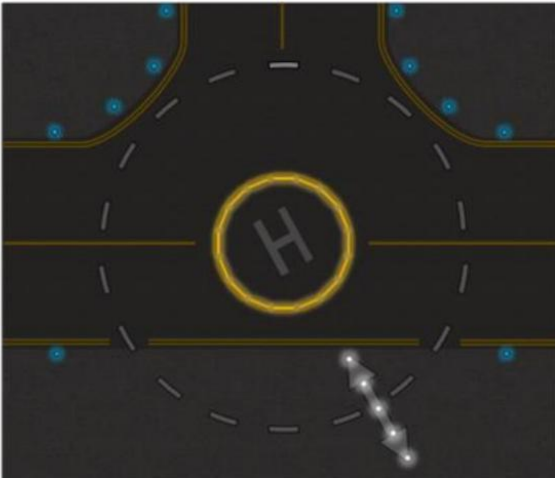
Figure 36: Lighting for FATOs on taxiways (source: CASA)
