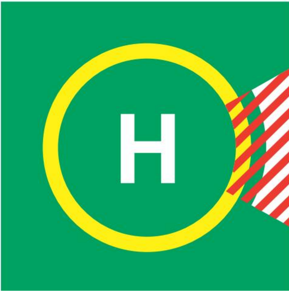
Figure 5-5. Helideck prohibited landing sector marking
