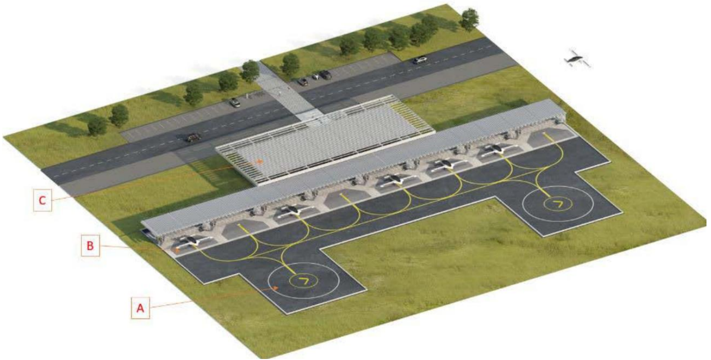
Figure 9. Lilium's urban vertiport layout with (a) takeoff area, (b) parking stands, and (c) terminal. Source: Lilium (2020)
