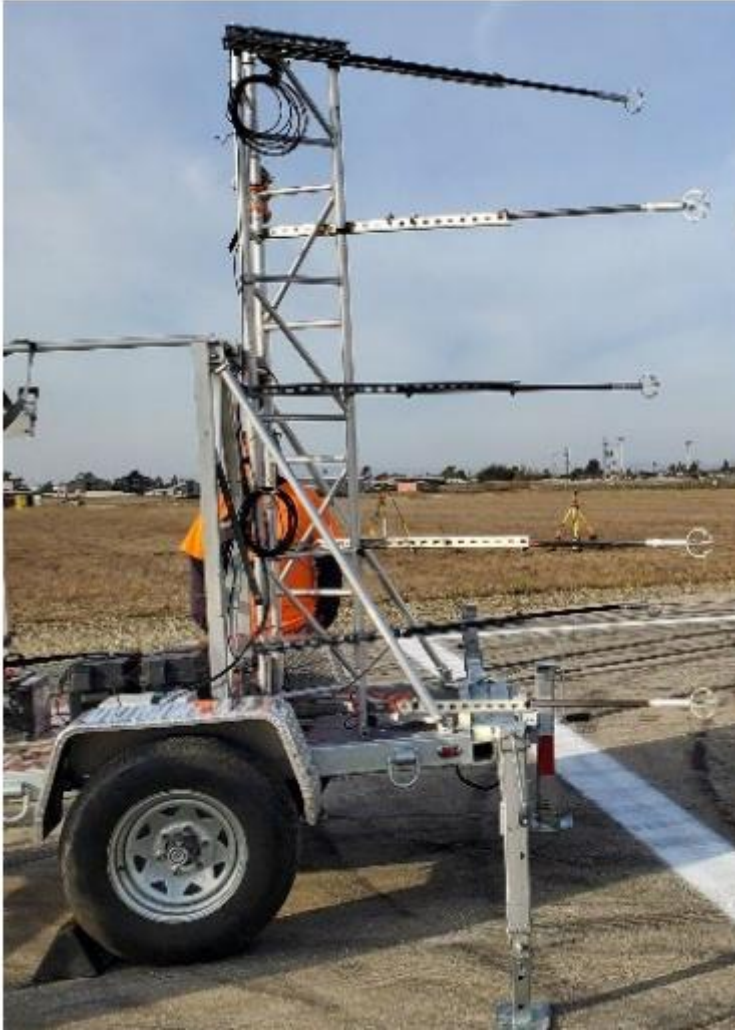
Figure 3. Vertical Array Mobile Cart
